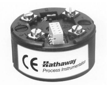
Hathaway T106 RTD Transmitter, Two Wire, Head Mounting, Features: Input from 100 ohm Pt. RTD, 1000 VAC Isolation, Linearized 4-20 mA Output, High Precision, High Accuracy and Performance Stability, Non-interactive Zero and Span Adjustments, Immunity from R.F. Interference, CE Conforming, Designed for Mounting in DIN B Heads, ISO 9001
