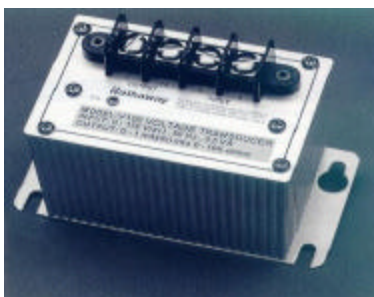
Hathaway AC Voltage Transducers, Standard Features: True RMS or Average-Sensing Models, 0.25% of full scale accuracy, 0.01% /°C temperature coefficient, 0.2%/year long-term stability, 2.5 kV transient immunity, 5 kV impulse test, 2 kV dielectric testing, Current and Voltage Outputs, ABS DIN rail mount or metal surface mount cases
