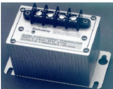
Hathaway AC Current Transducers, Standard Features: True RMS or Average-Sensing Models, 0.25% of full scale accuracy, 0.01% /°C temperature coefficient, 0.2%/year long-term stability, 2.5 kV transient immunity, 5 kV impulse test, 2 kV dielectric testing, Current and Voltage Outputs, ABS DIN rail mount or metal surface mount cases
