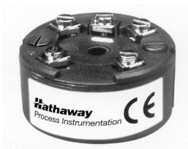
Hathaway T102P TC Transmitter, Computer Programmable, Features: Zero and Span Programmable Via Personal Computer, One Model for Both Type J & K, Linearized 4-20mA Output, High Accuracy and Performance Stability, Non-interactive Zero and Span Adjustments, Immunity from R.F. Interference, CE Conforming, Designed for Mounting on DIN B Heads, ISO 9001 Certified, Low Cost
