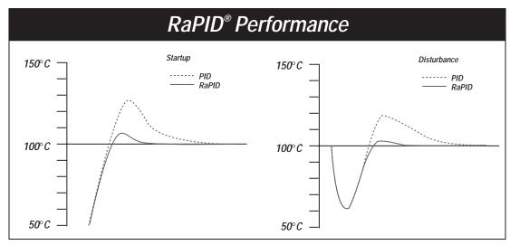
Results achieved against competitor PID and fuzzy logic controllers on a simulated load with two first order time constants of 80 and 30 seconds each, and a dead time of seven seconds.
