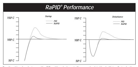
Results achieved against competitor PID and fuzzy logic controllers on a simulated load with two first order time constants of 80 and 30 seconds each, and a dead time of seven seconds.
